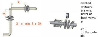
Tighten the flange screws crosswise regarding the torque required.
