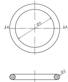
\* EPDM seals up to and including 54,0 mm installed as LBP seals ("leak before press"). Remaining seals as standard seals.
